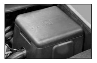
The underhood fuse/relay block is located near the battery in the engine compartment. See "Engine Compartment Overview" in the Index for more information on its location. Lift the cover for access to the fuse/relay block.
